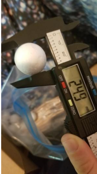
Figure 2 Me, measuring the diameter of the Styrofoam balls
