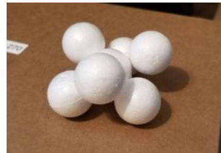
Figure 4 BCC model halfway finished
